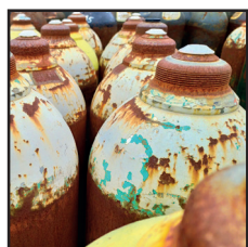
Rusty / Fatigued Cylinders
